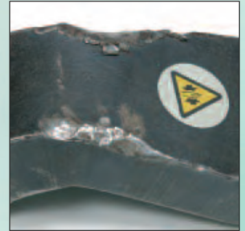
Signs of poor reaction are evident on this damaged foot. Reaction was taken at the wrong point on the foot and burring indicates that the foot was slipping off the reaction point.
